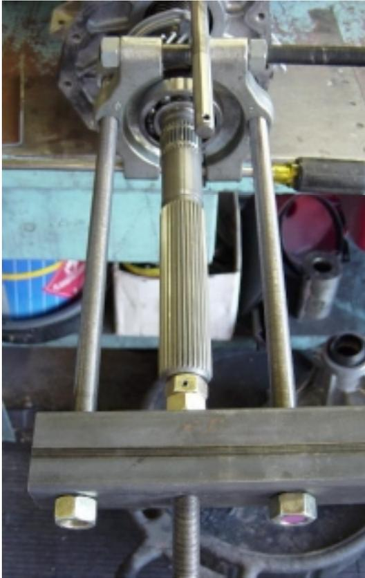
With the output shaft support bearing removed, remove the retaining ring, selectable thrust washer (it is a good idea to measure and record the thickness for reference), the reverse driven gear, needle bearing, and the bearing thrust washer.
