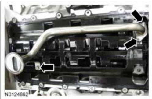
5. Tighten the oil pump screen and pickup tube-to-spacer bolt to 25 Nm (18 lb-ft).
