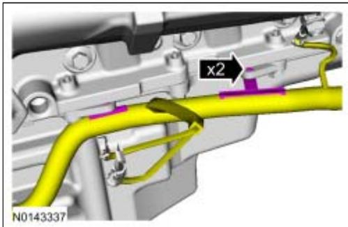
22. Disconnect the wire retainer. Remove the 2 nuts and the 2 wire harness retainer brackets from the oil pan stud bolts.
