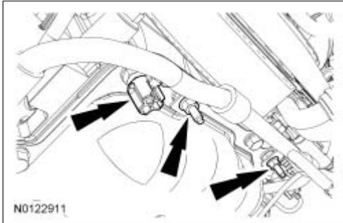
9. Attach the 2 wiring harness retainers to the oil pan.
