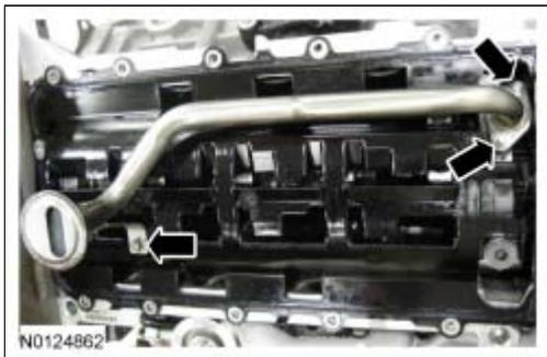
26. Remove and inspect the oil pan baffle and gasket, replace as necessary.
