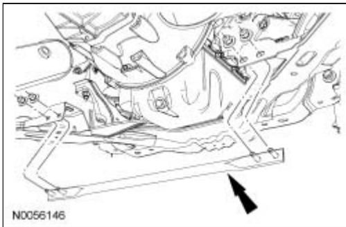
13. Remove the 9 screws and the lower air deflector.
