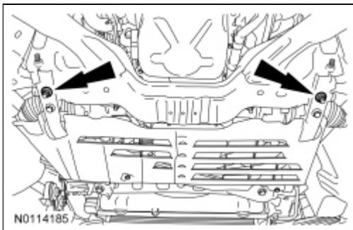
15. Remove the 6 bolts and remove the crossmember brace.
