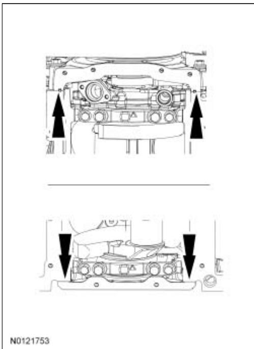
3. Position the oil pan baffle and gasket.
