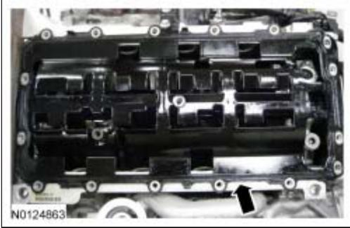
4. **NOTE:** The 2 oil pump screen and pickup tube-to-oil pump bolts must be tightened prior to tightening the oil pump screen and pickup tube-to-spacer bolt.
