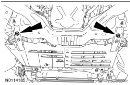
16. Install the lower air deflector and the 9 screws.
