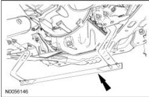
18. Using the Engine Support Bars, lower the engine onto the engine support insulators.
