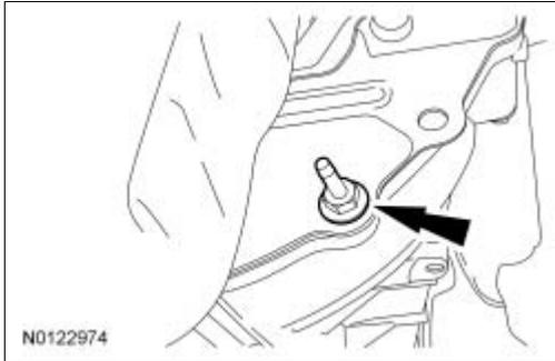
24. Remove the 13 bolts, the 3 stud bolts and the oil pan.
