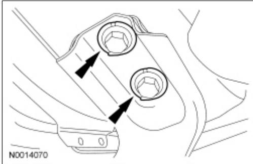
19. Remove the 4 subframe nuts and 4 subframe bolts.
