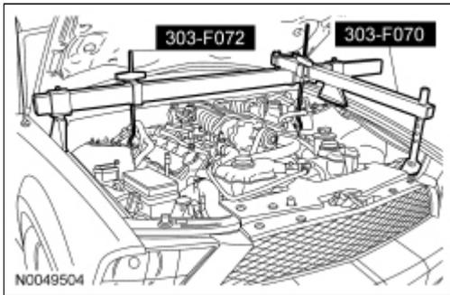
19. **NOTICE:** Do not tighten the engine support insulator nuts until the full weight of the engine is on the engine insulator or damage to the engine insulator may occur.
