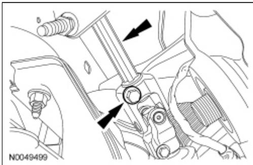
18. Mark the position of the 4 subframe nuts and 4 subframe bolts for referencing during assembly.
