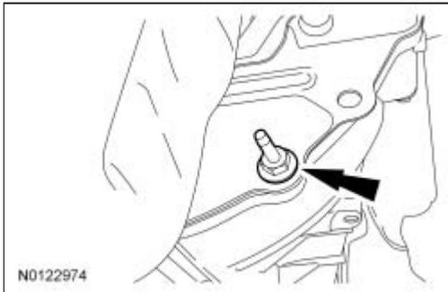
8. Install the 2 wire harness retainer brackets on the oil pan stud bolts and install the 2 nuts. Connect the wire retainer.
