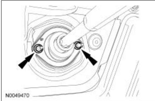
3. **NOTE:** Use a steering wheel holding device (such as Hunter® 28-75-1 or equivalent).
