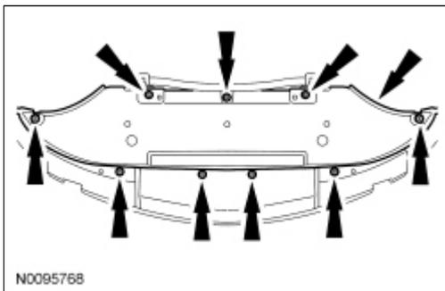
17. Install the subframe rear cross brace and the 4 nuts.
