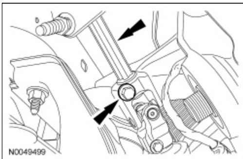
12. **NOTE:** Do not tighten the subframe nuts and bolts at this time.
