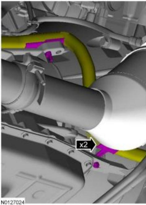
**RH HO2S on 5.0L engine with manual transmission**
