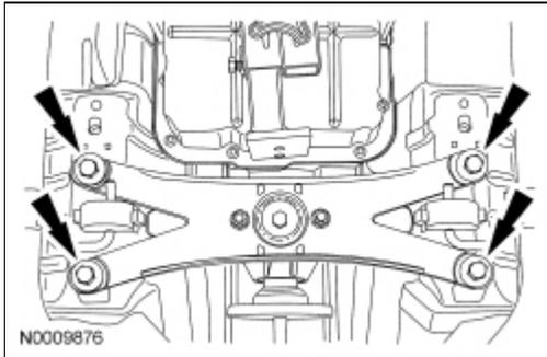
6. With the transmission support insulator neutralized, tighten the transmission support insulator bolt.
