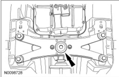
4. Remove the transmission crossmember bolts and remove the transmission crossmember.
