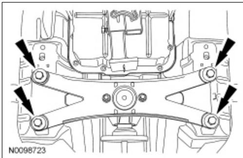
3. Loosely install the transmission support insulator bolt.
