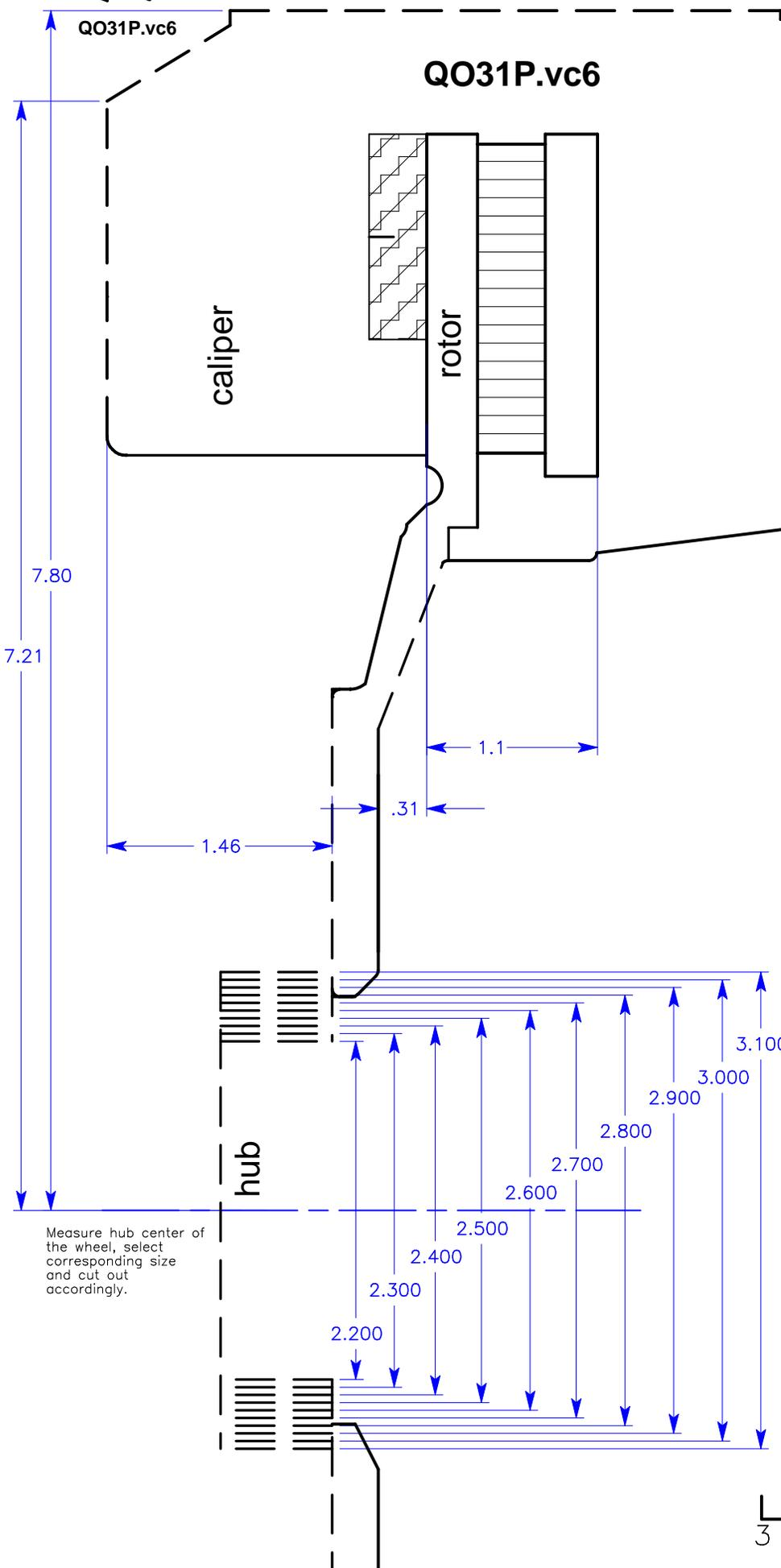
Because of the abundance of wheel companies and styles, it is impossible for Baer Racing to guarantee fit of their brake systems into a specific wheel style and/or manufacturer. To aid in determining for yourself if your wheels are likely to fit around a specific Baer Racing brake upgrade, we supply this brake system template. To use this template to determine fit, follow these simple instructions.
