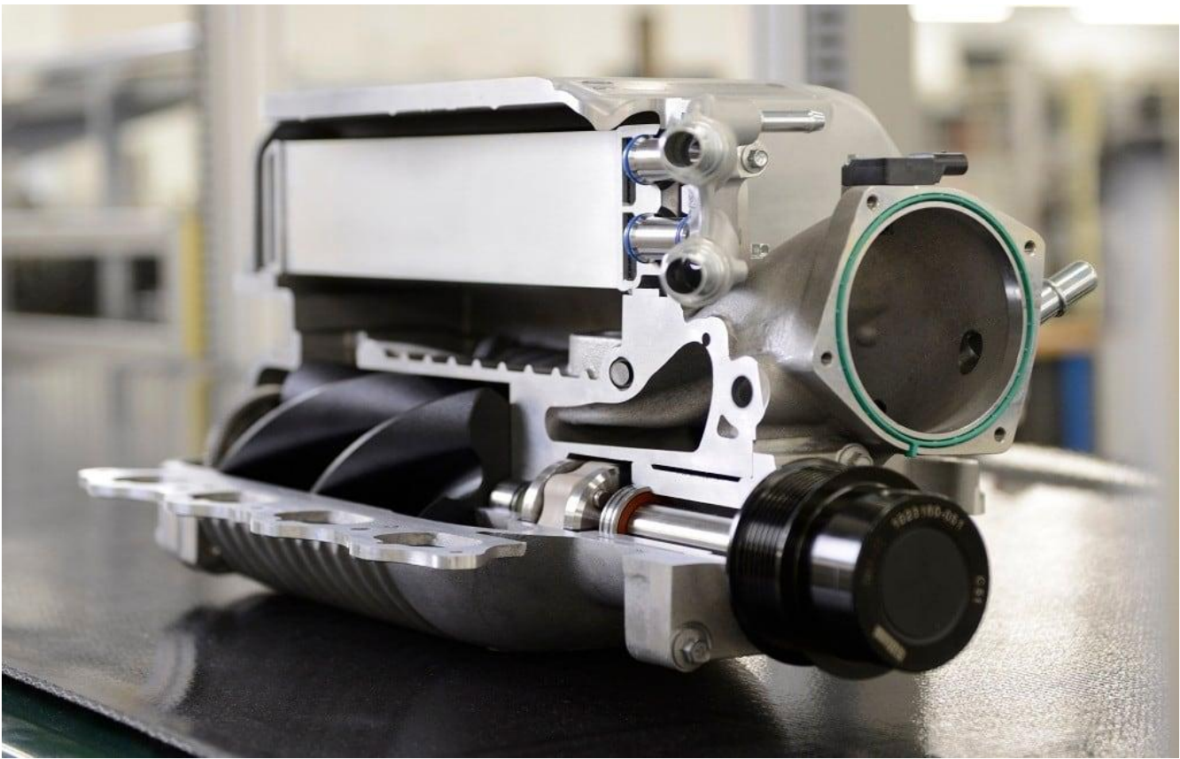
Supercharger cutaway
